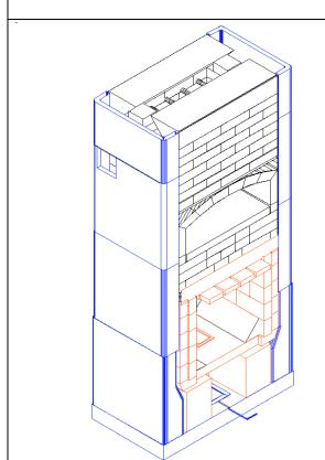
View of core, showing location of 6x6 notch for bypass damper.
