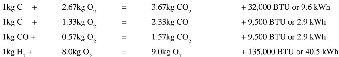
Once the chemical composition of a fuel is known, the above formulas can be used to calculate the heat content.
