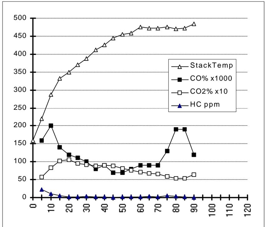
**Figure 1. Flue gas analysis curves for a 1½ hr test run**
