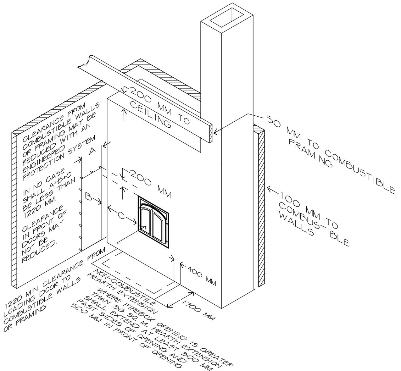
**Figure 5. ASTM clearances to combustibles for masonry heaters**
