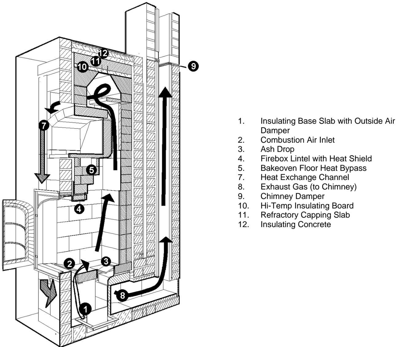
Figure 3. Cutaway illustration of a contraflow heater.
