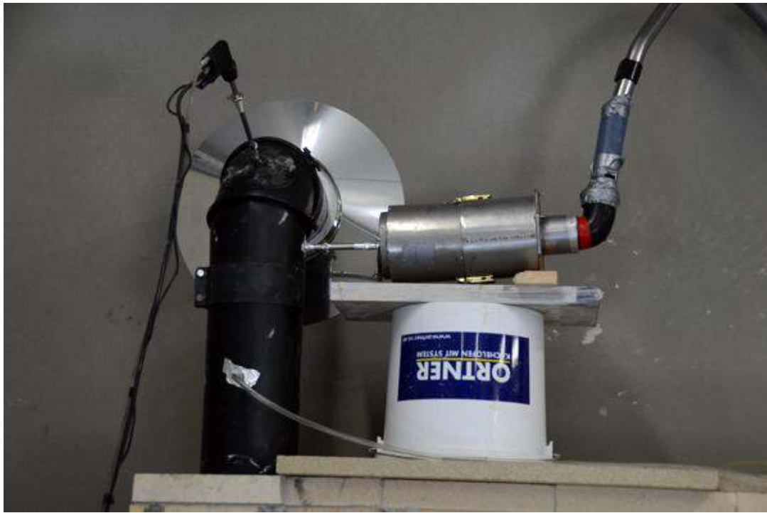
Testing set-up for the double-bell heater version. Probe from the NOVA on the left, Condor on right.
