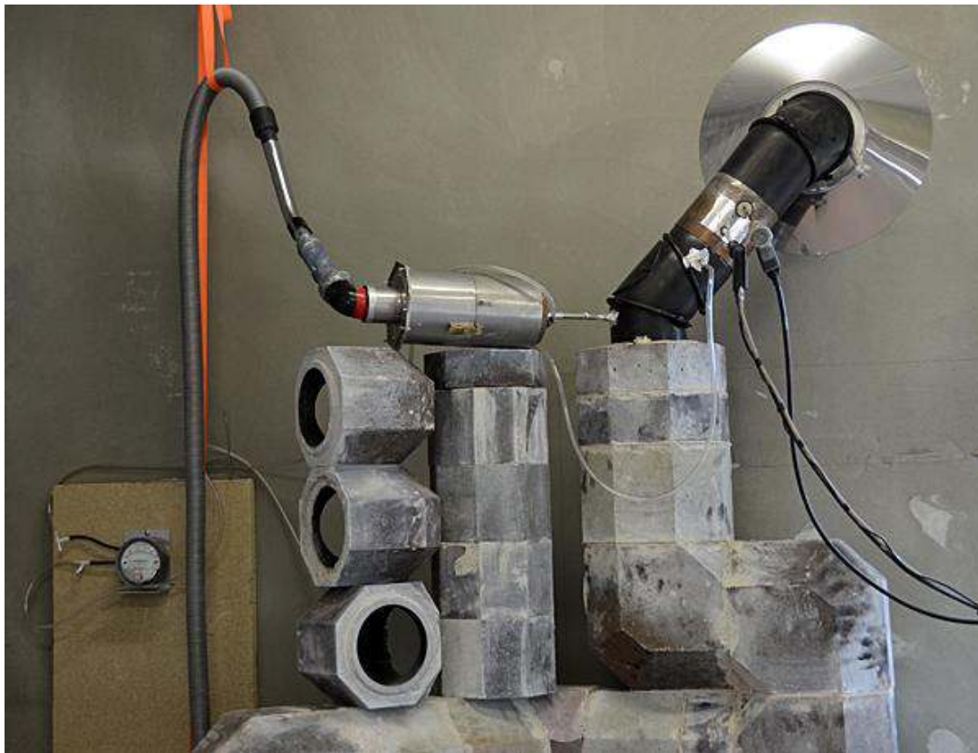
KMS version testing set-up. Probes from NOVA and TESTO on the right, Condar with Magnehelic on the left.
